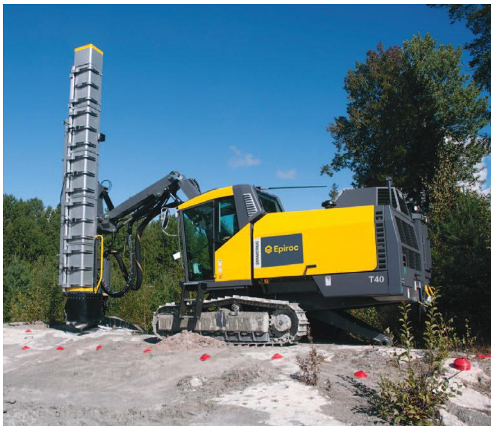
The Noise Reduction Kit is able to reduce the volume of drilling and rod changes by approximately 10 decibels.
